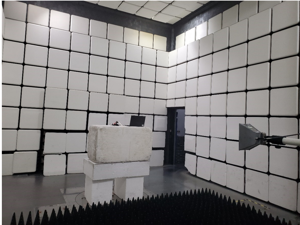
Picture 1 Radiated Emission Test Setup
