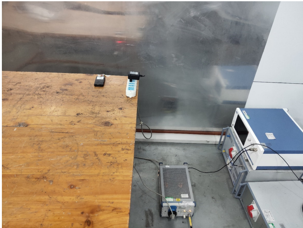
Picture 2 Conducted Emission Test Setup
