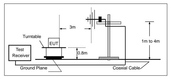
(c) For radiated emissions above 1000MHz
