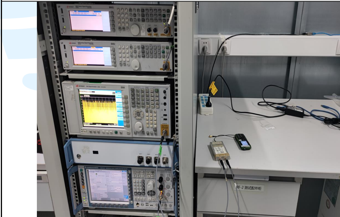
RF Conducted Test Setup
