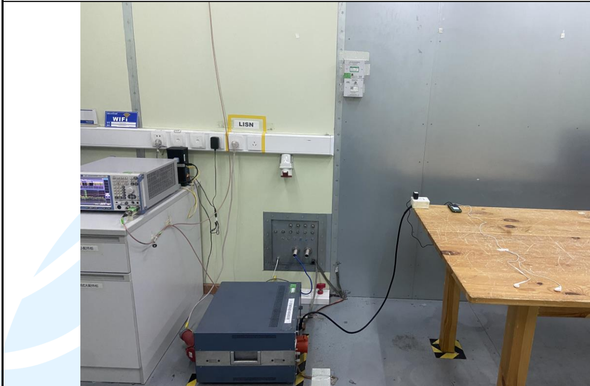
Conducted Emission Test Setup
