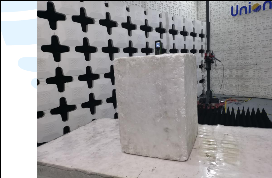
Radiated emission Test Setup (Above 1 GHz)
