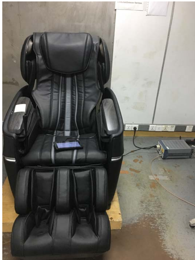
Photograph of set-up for conducted Emission
