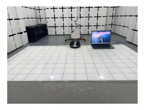
Set-up for Radiated Spurious Emission, Above 1GHz
