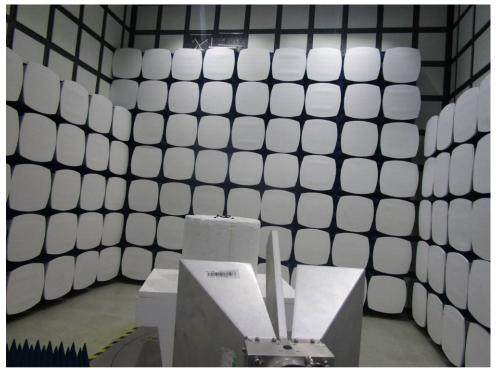
1.3 Radiated Spurious Emissions Test Setup
