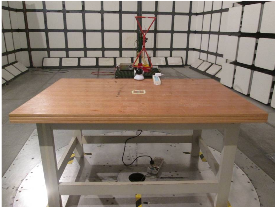
Radiated Emissions – Front View (30-1000 MHz)
