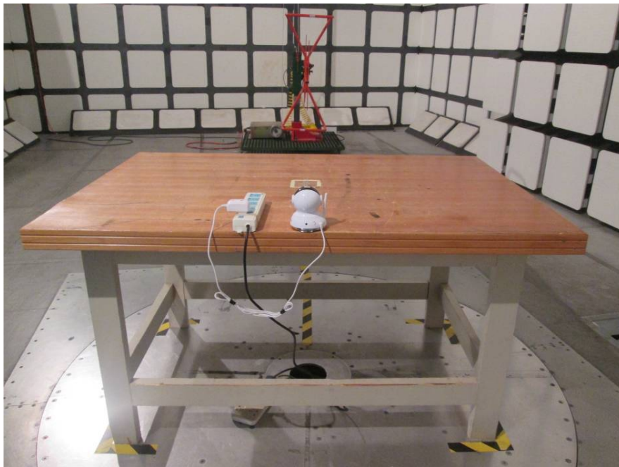
Radiated Emissions – Rear View (30-1000 MHz)
