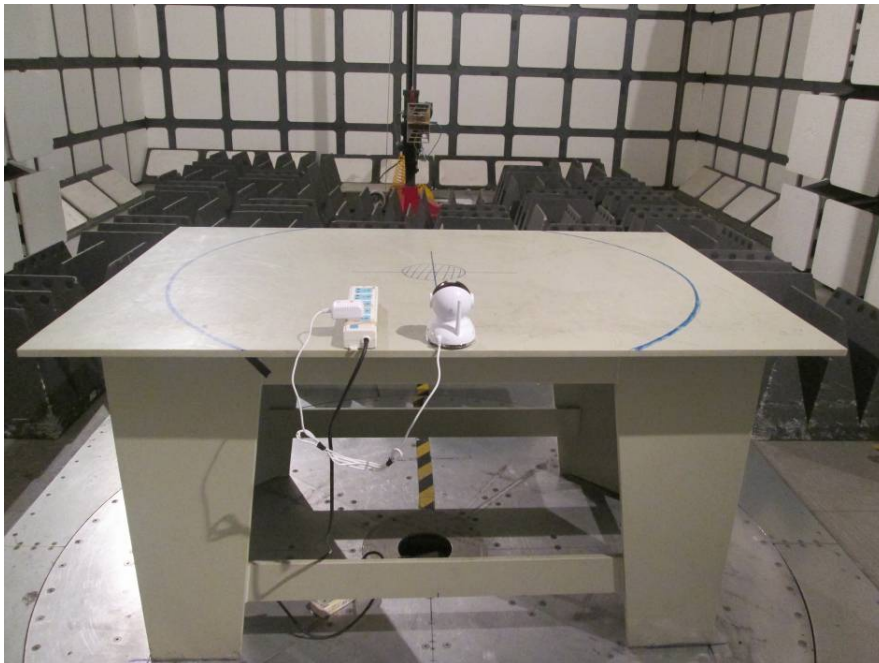
Radiated Emissions – Rear View (1-25 GHz)
