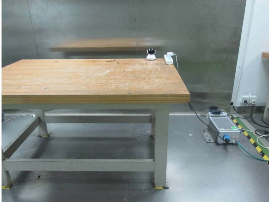
Conduction Emissions - Front View
