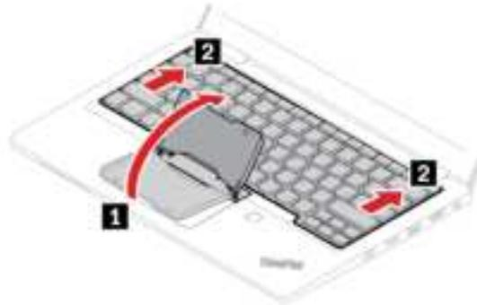
7. Pivot the keyboard slightly upward **1** and then turn over the keyboard **2**.
