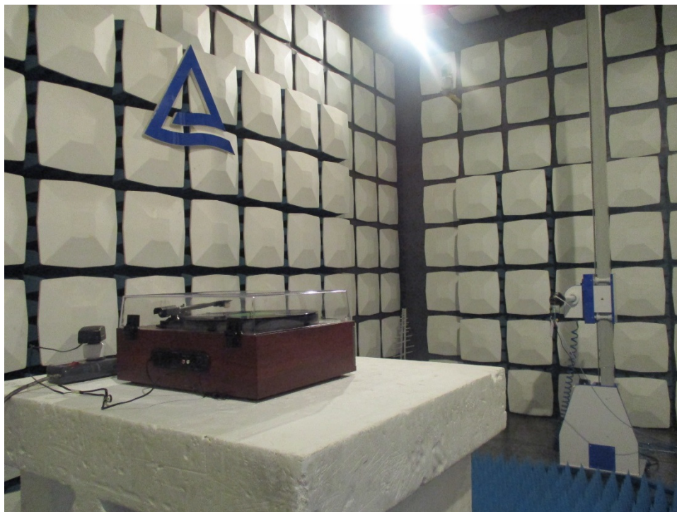
Photograph 4: Set-up for Radiated Spurious Emission, 18GHz - 26.5GHz
