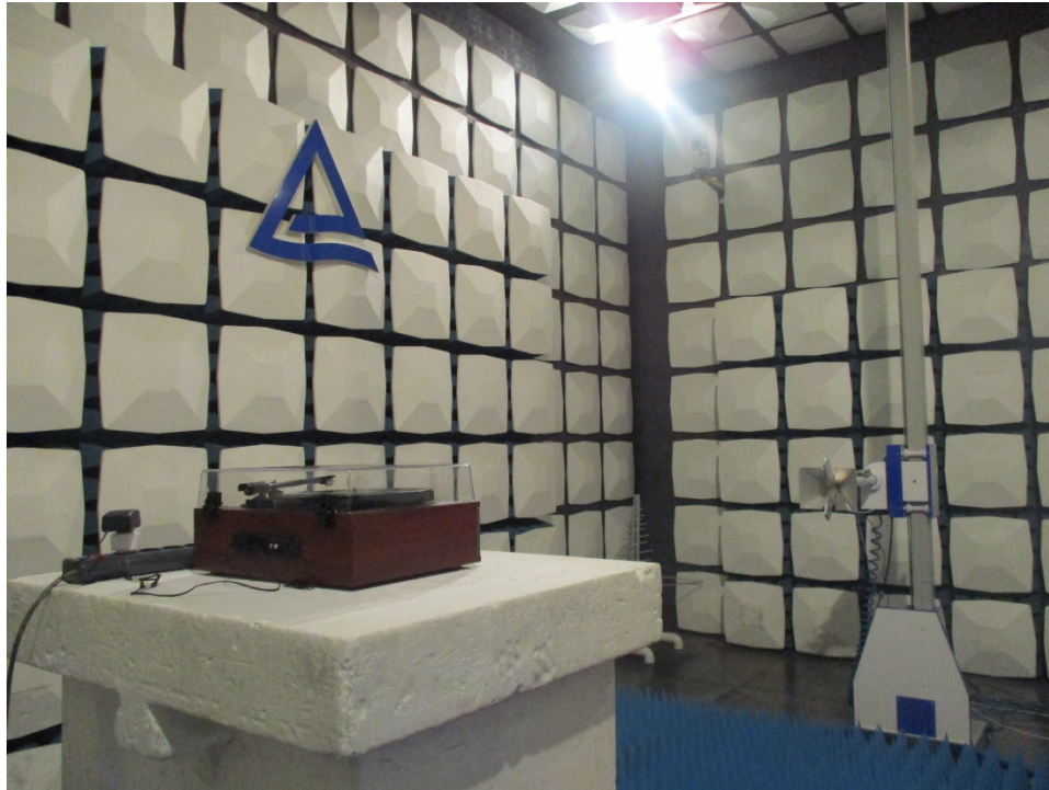
Photograph 3: Set-up for Radiated Spurious Emission, 1GHz - 18GHz
