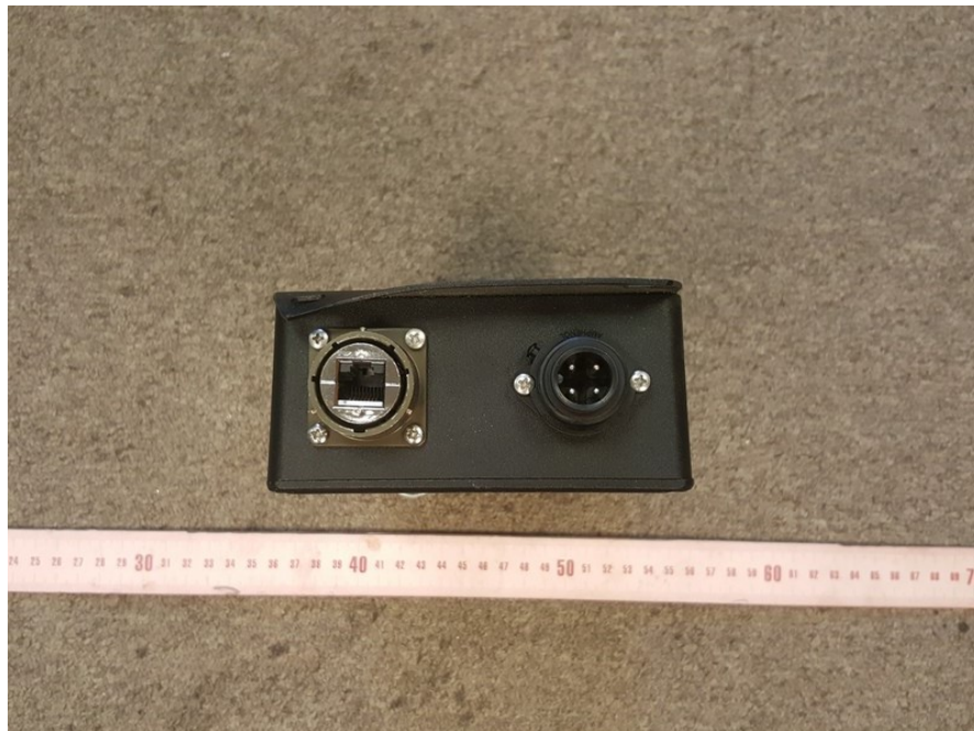
Cable Interface_ Network Port Side
