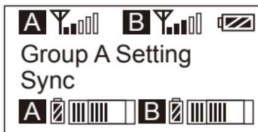
6.2 Long press
