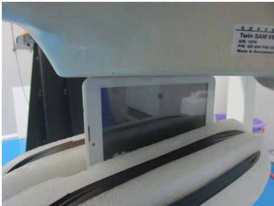
Body Worn Right Setup Photo(0mm)
