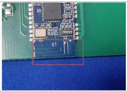
The antenna is PCB antenna.
