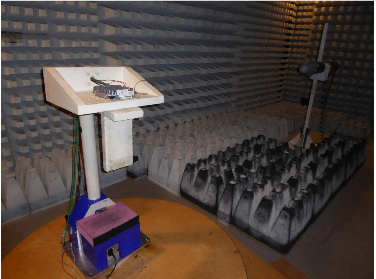
Test setup fully anechoic chamber (1 – 12 GHz)
