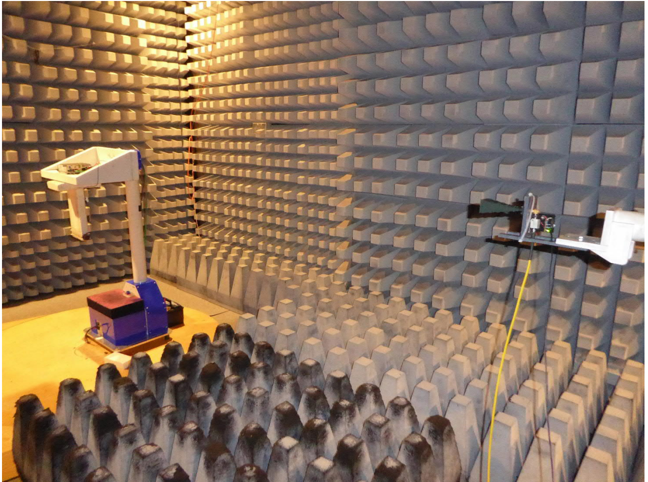
Test setup fully anechoic chamber (18 – 26.5 GHz)
