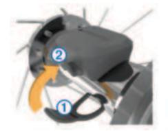
The sensor may be tilted when installed on an asymmetrical hub. This does not affect operation.
