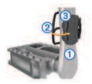
**4** Rotate the crank arm to check for clearance.
