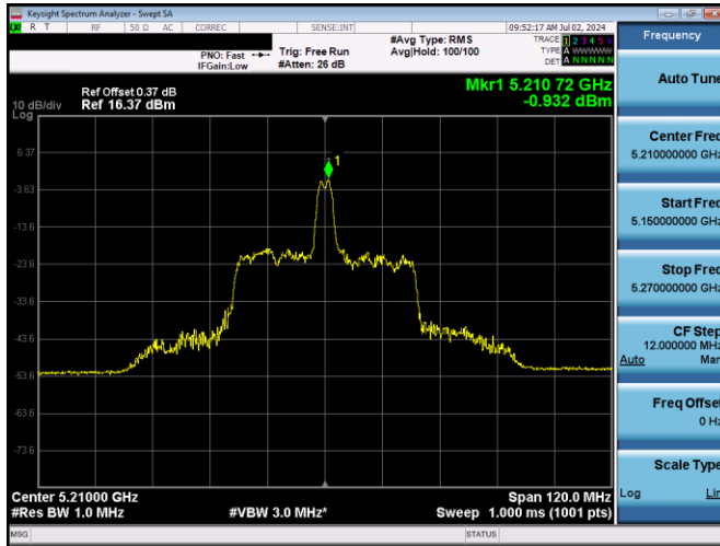
Plot 7-385. ISSED PSD SDM Antenna WF5T (80MHz BW 11ax Index 18 - RU26 - Ch.42)
