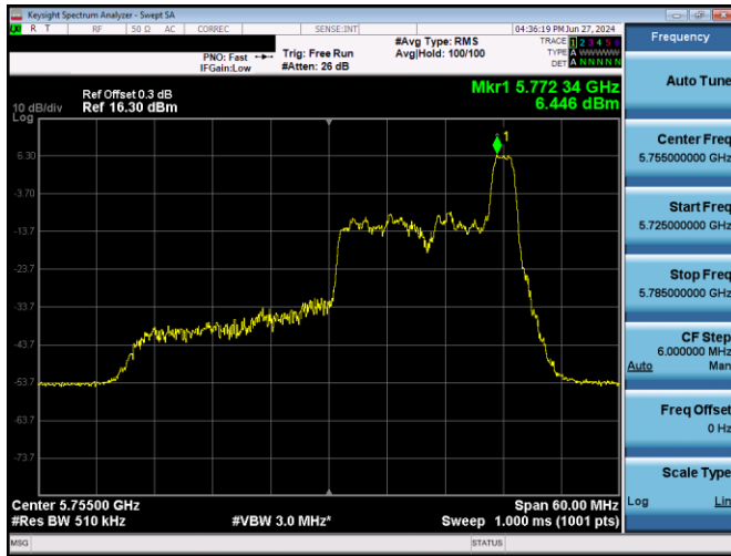
Plot 7-355. PSD CDD Antenna WF5T (40MHz BW 11ax Index 17 - RU26 - Ch.151)
