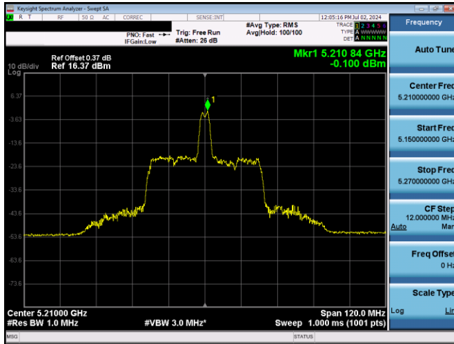
Plot 7-386. ISSED PSD SDM Antenna WF2 (80MHz BW 11ax Index 18 - RU26 - Ch.42)
