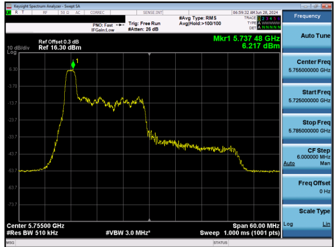
Plot 7-352. PSD CDD Antenna WF2 (40MHz BW 11ax Index 0 - RU26 - Ch.151)
