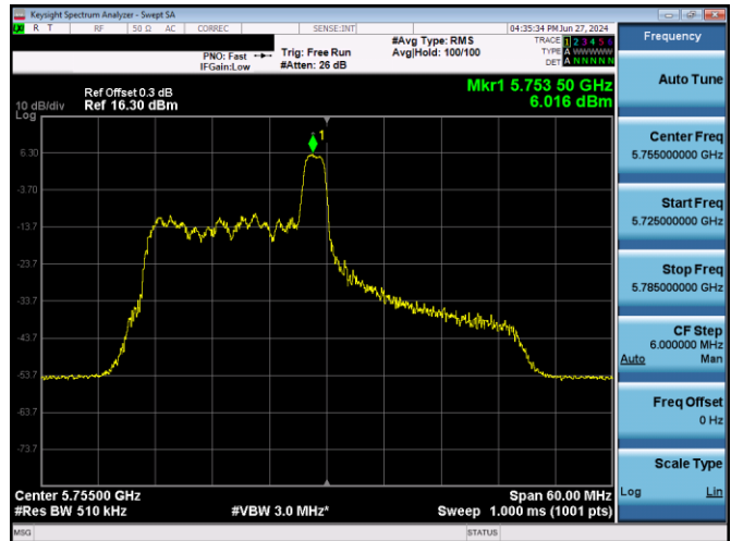
Plot 7-353. PSD CDD Antenna WF5T (40MHz BW 11ax Index 8 - RU26 - Ch.151)
