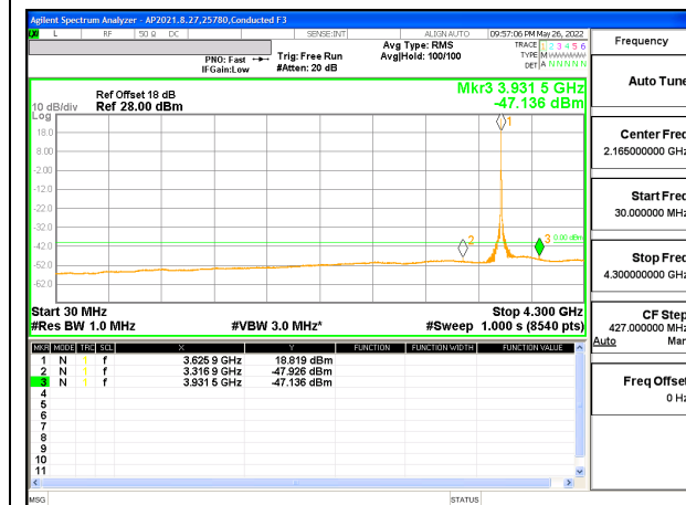
LTE B48 20MHz + 20MHz QPSK Middle Ch RB1-99 + RB1-0 (30MHz to 4.5GHz)
