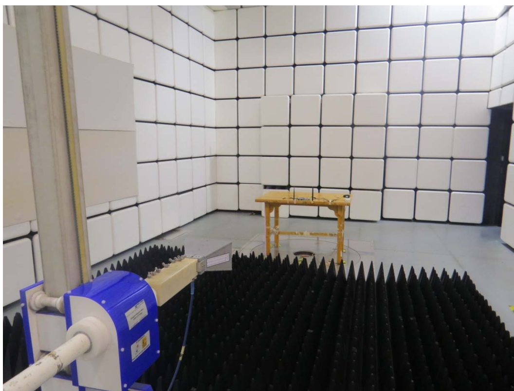
Picture 2: Radiated Spurious Emissions Test setup
