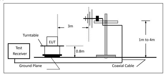
(c) For radiated emissions above 1000MHz
