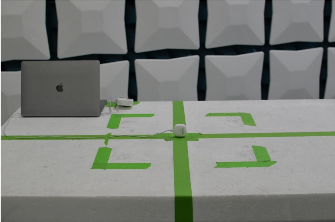
Figure 19: 30MHz-1GHz Test Setup (Front View)
