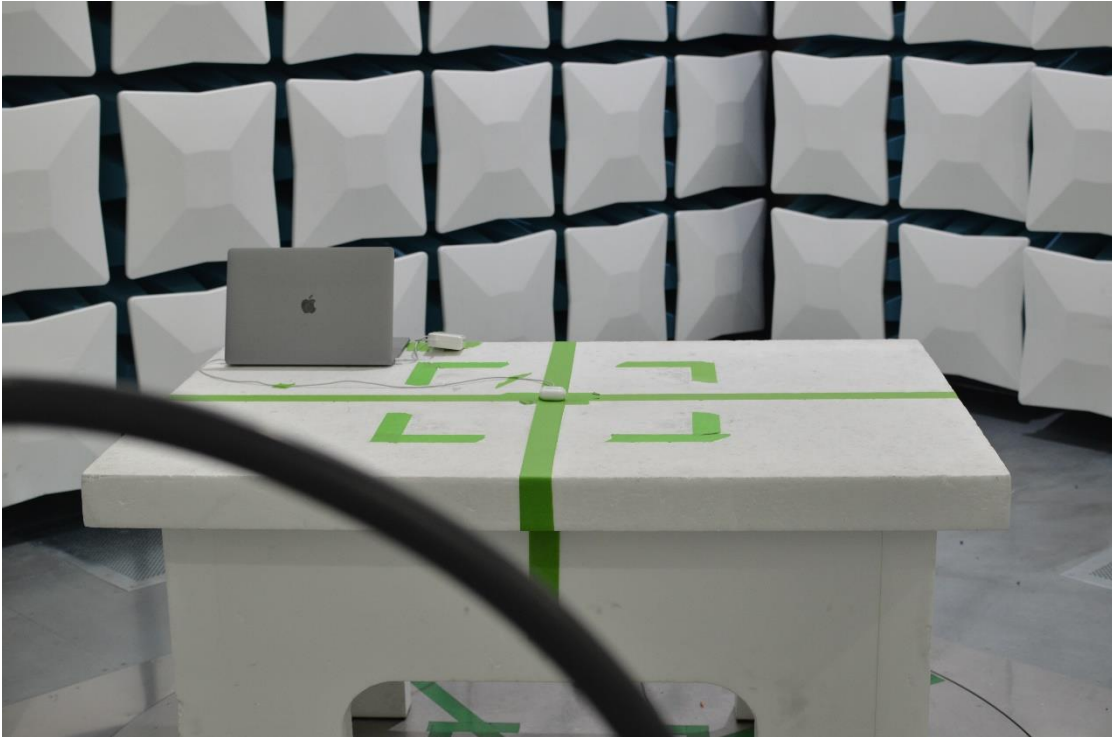
Figure 23: 9kHz-30MHz Test Setup (Front View)
