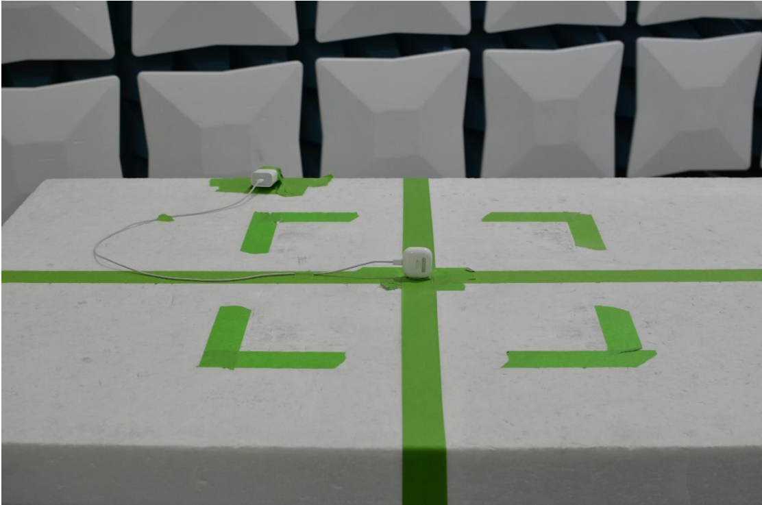
Figure 13: 30MHz-1GHz Test Setup (Front View)
