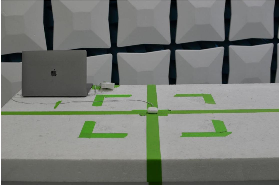
Figure 17: 30MHz-1GHz Test Setup (Front View)
