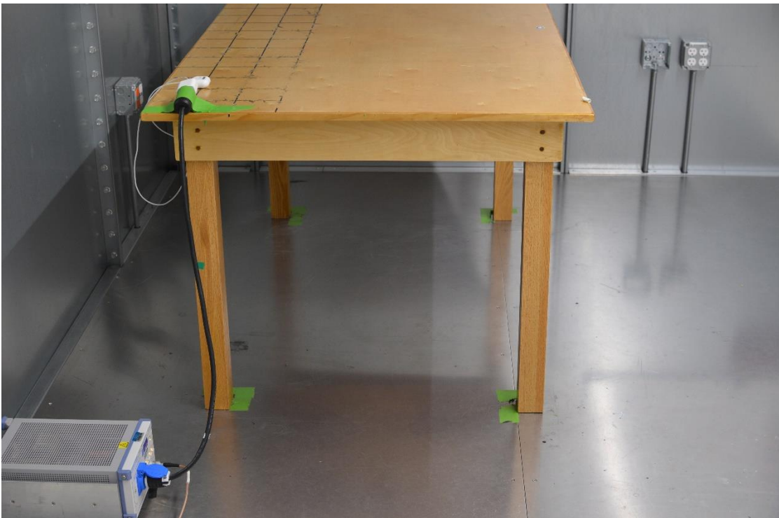
Figure 2: AC Line Conducted Emissions (Side View)
