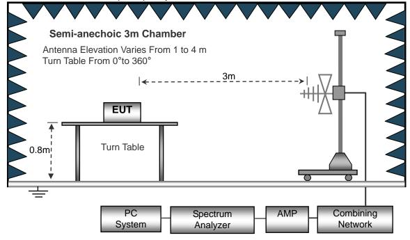
(C) Radiated Emission Test-Up Frequency Above 1GHz
