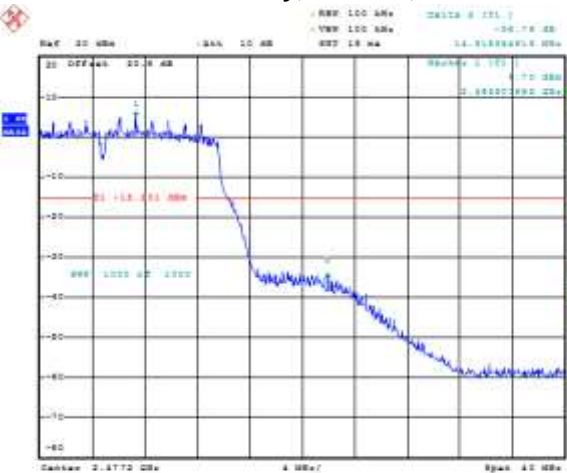
Figure 6-24: Band Edge Compliance Secondary, 802.11n, Channel 11, MCS 0
