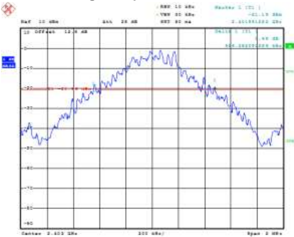
Figure 5-1: 20 dB Bandwidth Single freq. CH 0 Static PBRS, DH5
