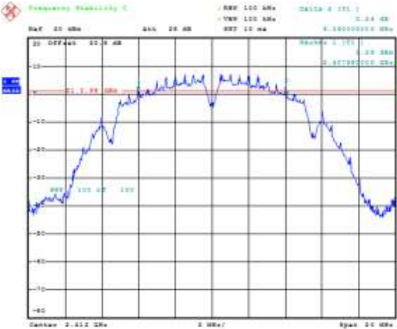
Figure 6-1: 6 dB Bandwidth Primary, 802.11b, Channel 1, 1 Mbps
