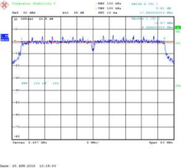
Figure 6-6: 6 dB Bandwidth Primary, 802.11g, Channel 11, 6 Mbps
