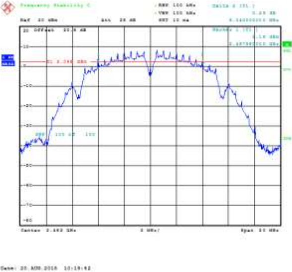
Figure 6-7: 6 dB Bandwidth Primary, 802.11n, Channel 1, MCS 0
