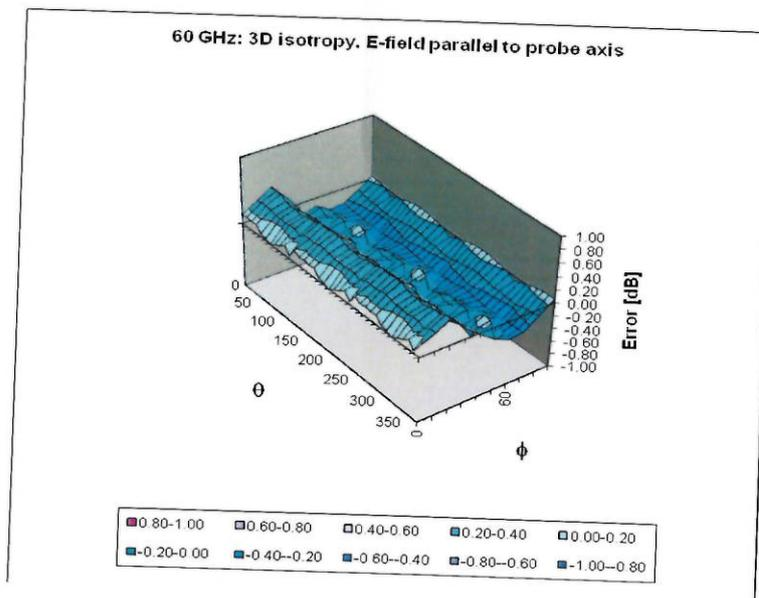
Probe isotropy for  $E_{tot}$ : probe rotated  $\phi = 0^\circ$  to  $360^\circ$ , tilted from field propagation direction  $\vec{k}$
