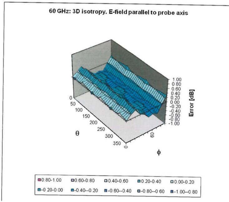
Probe isotropy for  $E_{tot}$ : probe rotated  $\phi = 0^\circ$  to  $360^\circ$ , tilted from field propagation direction  $\vec{k}$
