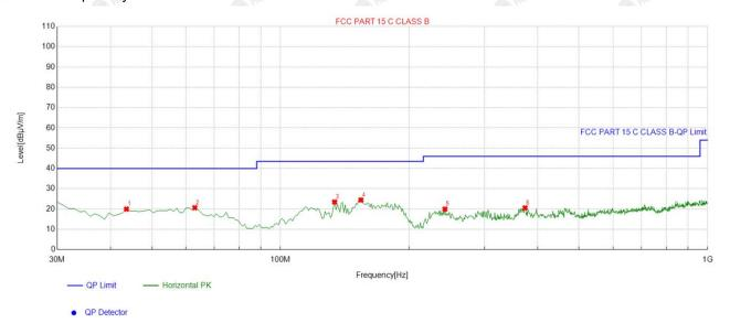
Suspected List Freq. Factor Reading Level Limit Margin Height Angle NO. Polarity [MHz] [dB]  $[dB\mu V/m]$  $[dB\mu V/m]$  $[dB\mu V/m]$ [dB] [cm] [°] 43.593594 -13.30 19.98 40.00 20.02 100 236 Horizontal 33.28 63.013013 -14.48 35.11 20.63 40.00 19.37 100 2 Horizontal 133.89389 -17.40 3 40.89 23.49 43.50 20.01 100 340 Horizontal 154.28428 -17.76 42.23 24.47 43.50 19.03 100 340 Horizontal 242.64264 -13.42 33.40 19.98 46.00 26.02 100 328 Horizontal
