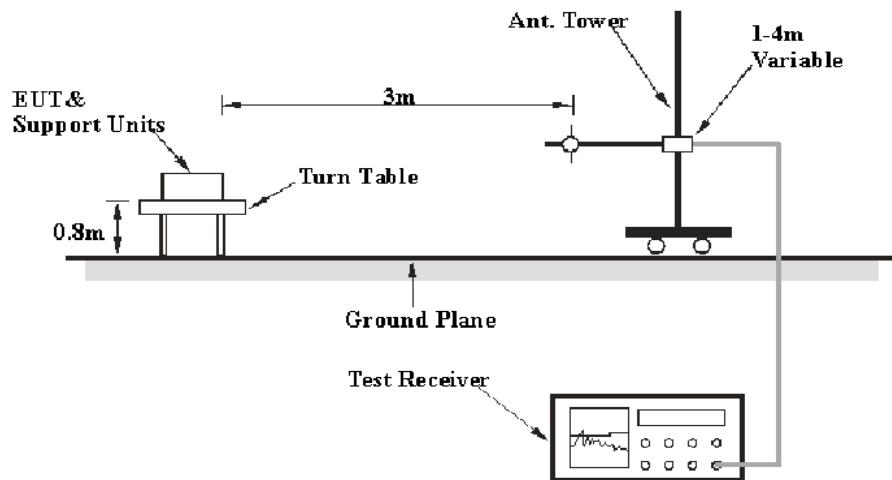
The radiated emission tests were performed in the 3 meters, using the setup accordance with the ANSI ANSI C63.10-2013. The specification used was the FCC 15.209 and FCC 15.247 limits.
