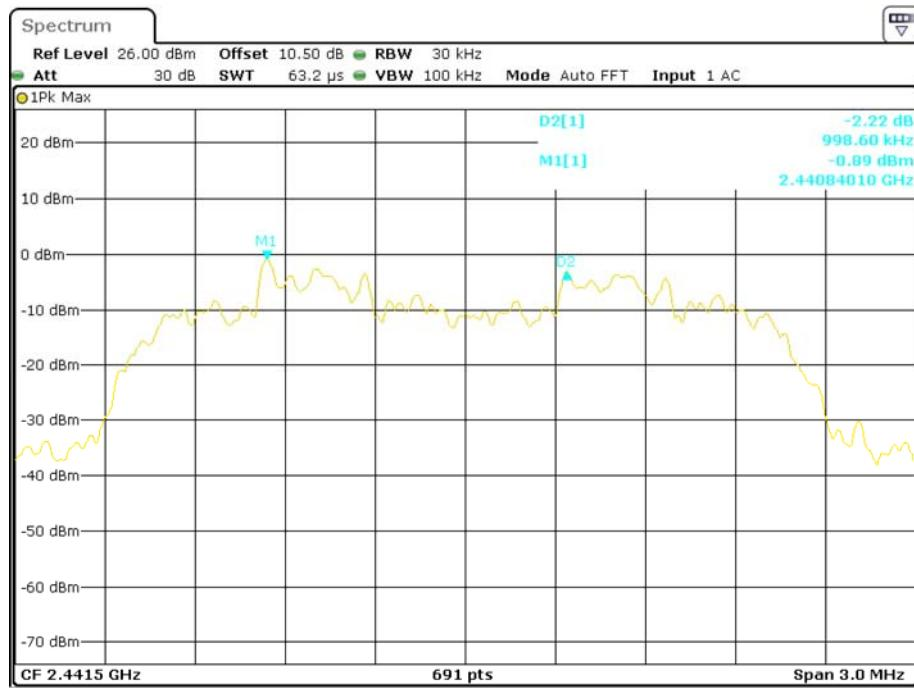
**EDR ( $\pi/4$ -DQPSK): High Channel**
