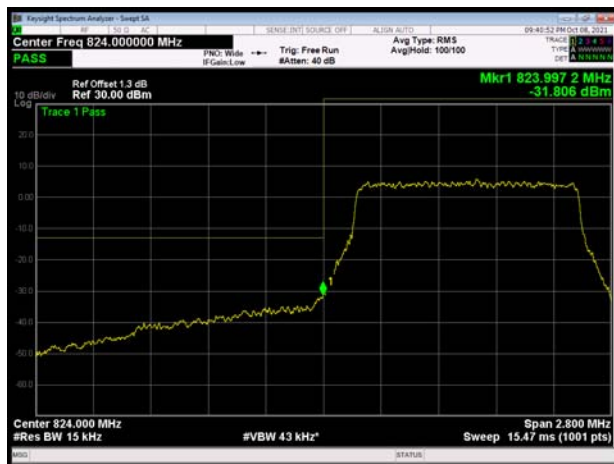
LTE Band 5 16QAM 3MHz CH-Low 1RB
