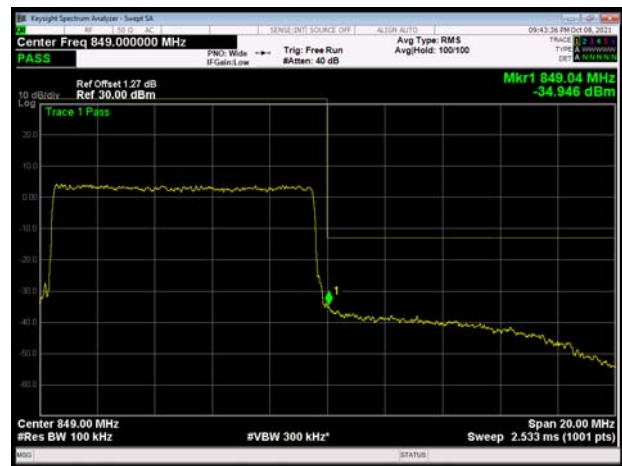
LTE Band 5 64QAM 1.4MHz CH-High 1RB
