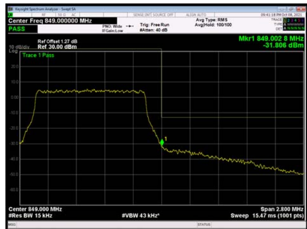
LTE Band 5 16QAM 3MHz CH-High 1RB
