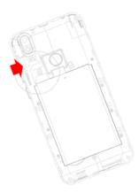
Insert the battery by aligning the metal contacts on the battery with the metal contacts in the battery compartment. Gently push down on the battery until it clicks into place.
