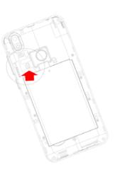
3. Hold the SIM card with the cut corner oriented as shown and slip them into the card slots.
