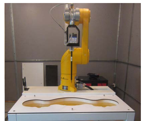
Figure 4.1 DASY5 Test System
