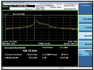
NB-IoT Band 13 BPSK 3.75KHz 1@0 CH-Middle
