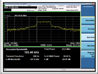
NB-IoT Band 13 QPSK 15KHz 12@0 CH-High
