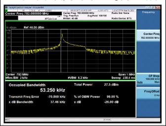
NB-IoT Band 13 QPSK 15KHz 1@0 CH-Middle
