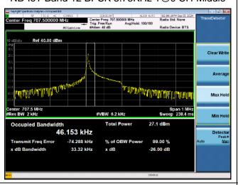
NB-IoT Band 12 BPSK 15KHz 1@0 CH-Middle
