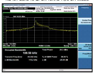
NB-IoT Band 13 QPSK 3.75KHz 1@0 CH-High
