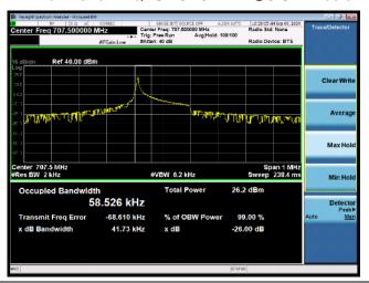
NB-IoT Band 12QPSK 15KHz 1@0 CH-Middle
