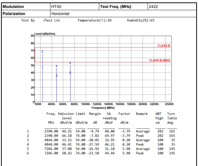
Note 1: Emission Level (dBuV/m) = SA Reading (dBuV) + Factor\* (dB/m)
