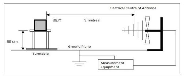
Test Sample: Enterprise Radio Module FCC Part 15.247 ANSI C63.4-2014
