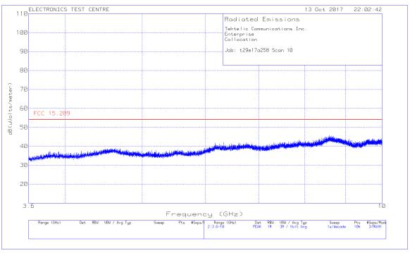
Test Sample: Enterprise Radio Module FCC Part 15.247 Report #: t29e17a258-FCC
