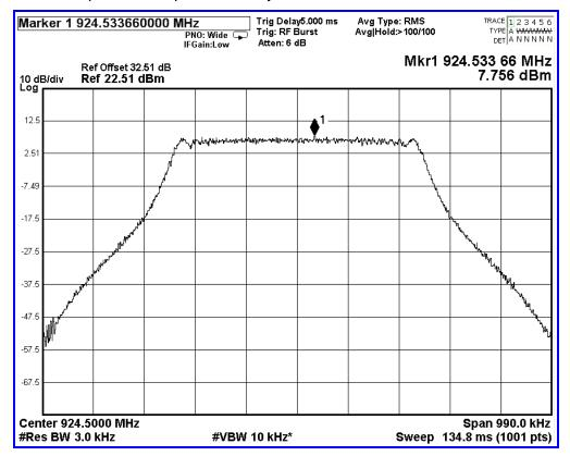
Screen Capture from spectrum analyzer: Antenna 1: 1 Carrier, 925.1 MHz
