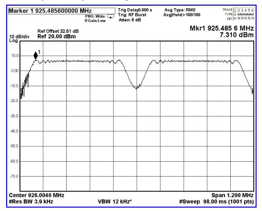
Screen Capture from spectrum analyzer: Antenna 2: 2 Carrier, 926.3 MHz & 925.7 MHz
