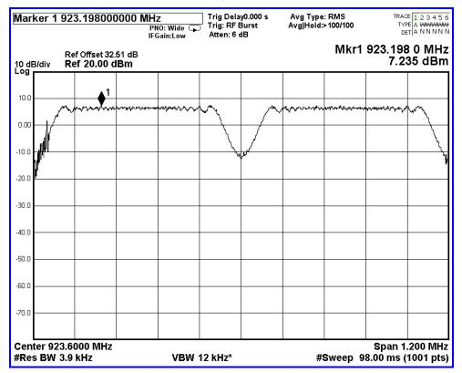
Screen Capture from spectrum analyzer: Antenna 1: 2 Carrier, 923.9 MHz w/ 923.3 MHz
