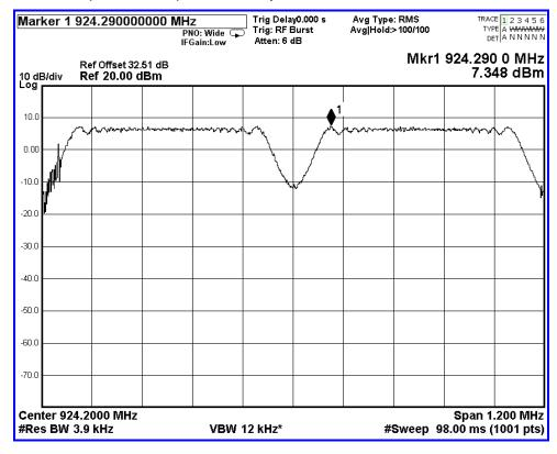
Screen Capture from spectrum analyzer: Antenna 2: 2 Carrier, 924.5 MHz w/ 925.1 MHz
