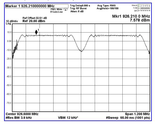
Screen Capture from spectrum analyzer: Antenna 2: 2 Carrier, 926.9 MHz w/ 926.3 MHz
