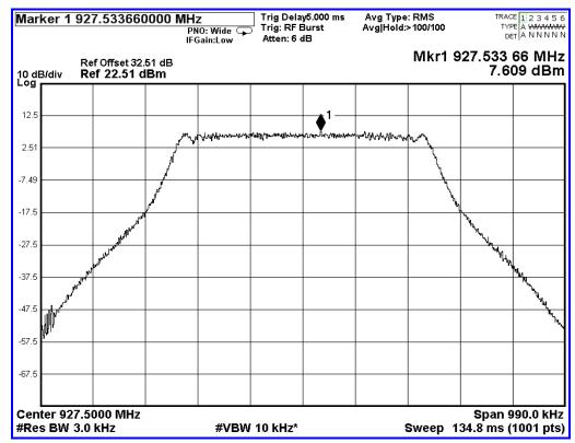
Screen Capture from spectrum analyzer: Antenna 1: 2 Carrier, 923.3 MHz w/ 923.9 MHz
