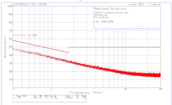
Plot of Radiated Emissions: Measuring Antenna 2<sup>nd</sup> Orientation
