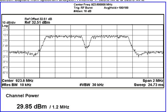
Screen Capture from spectrum analyzer: Antenna 1: 923.9 MHz & 924.5 MHz
