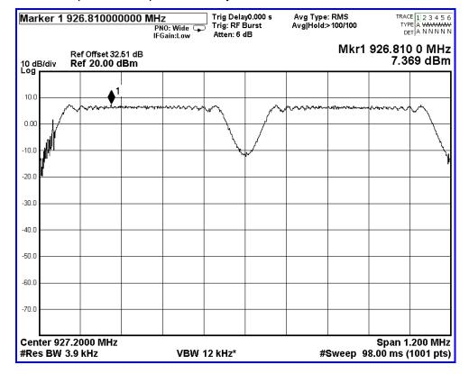
Screen Capture from spectrum analyzer: Antenna 2: 2 Carrier, 927.5 MHz & 926.9 MHz
