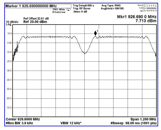
Screen Capture from spectrum analyzer: Antenna 2: 2 Carrier, 926.9 MHz & 927.5 MHz
