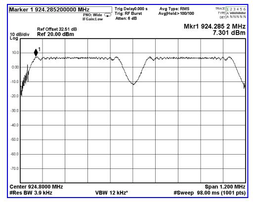
Screen Capture from spectrum analyzer: Antenna 2: 2 Carrier, 925.1 MHz w/ 924.5 MHz
