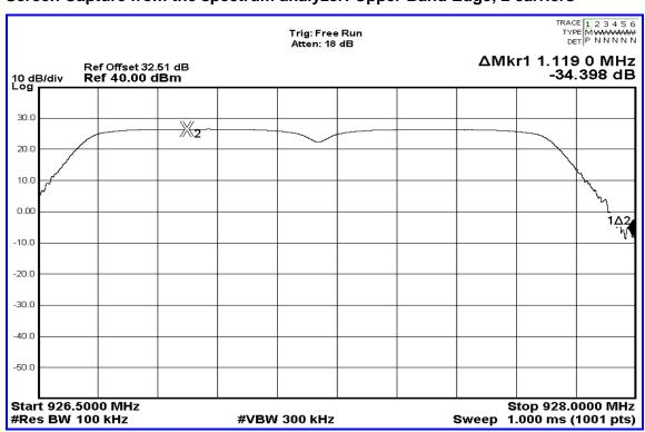
Test Sample: Enterprise Radio Module FCC Part 15.247
