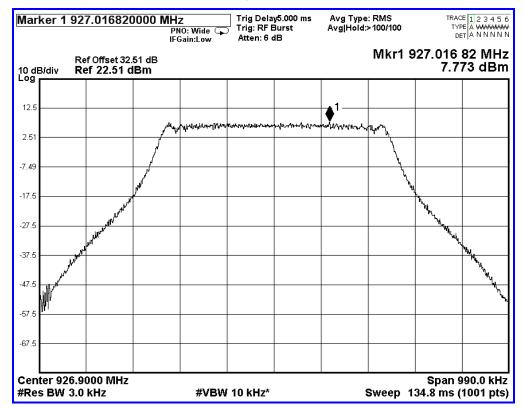
Screen Capture from spectrum analyzer: Antenna 2: 1 Carrier, 927.5 MHz
