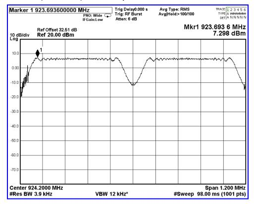
Screen Capture from spectrum analyzer: Antenna 1 2 Carrier, 924.5 MHz w/ 923.9 MHz
