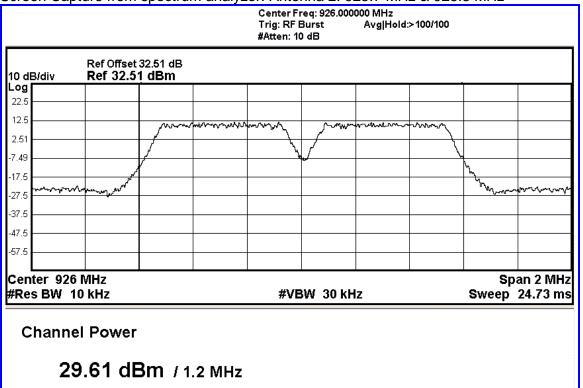
Screen Capture from spectrum analyzer: Antenna 2: 926.3 MHz & 926.9 MHz
