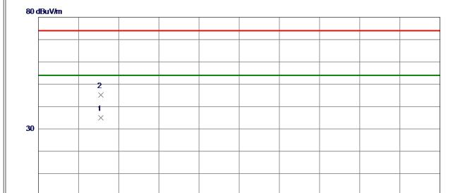
Reading Correct Measure Limit No. Freq. Margin Level Factor ment MHz dBuV/m dB dBuV/m dBuV/m dB Detector Comment 1 \* 4959. 9760 30. 11 4.81 34.92 54.00 -19.08AVG 4959. 9930 40. 35 4.81 45. 16 74.00 -28.84Peak
