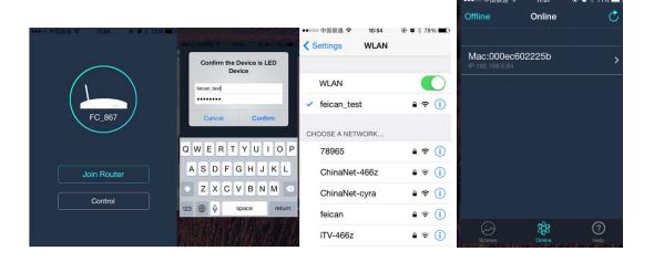
4.If the controllers successfully connect your router and the device will become a client state, then the signal FC -XXX will disappear in WLAN. If you find FC\_XXX signals in the list of mobile phones WLAN. it will testify the device is restored to factory condition, so you need to connect router with device again. Pay attention: After the device is powered off then power on again, the device will connect to the router before connected automatically. The following
