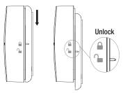
Decide upon your placement position and attach the Bracket (J) with either Screws (KK) or preinstalled double-sided adhesive tape.
