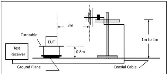
(c) For radiated emissions above 1000MHz
