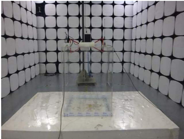
Radiated Spurious Emissions Test Setup Below 1GHz
