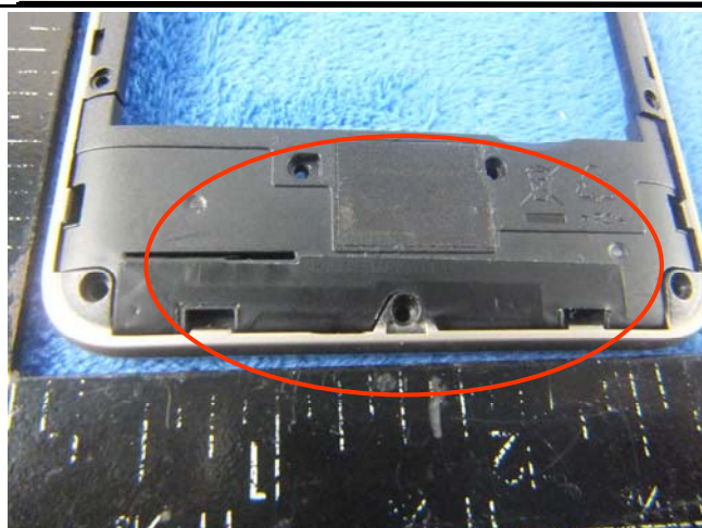
UMTS-FDD/GSM Antenna View
