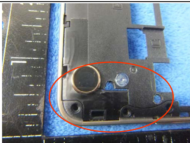
LTE - Antenna View
