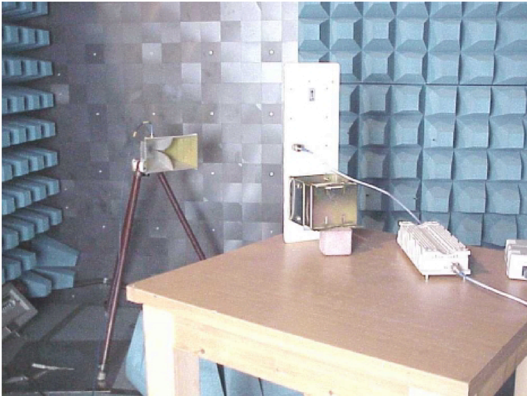
Photo #5 Radio unit with MTI sector antenna P/N MT-484025/NV. Spurious emission test
