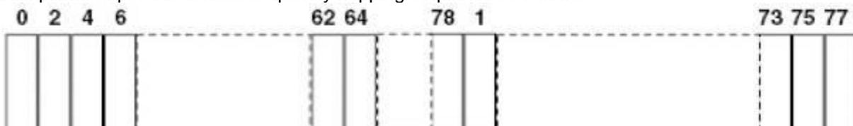
Each frequency used equally on the average by each transmitter. The system receiver have input bandwidths that match the hopping channel bandwidths of their corresponding transmitter and shift frequencies in synchronization with the transmitted signals.
