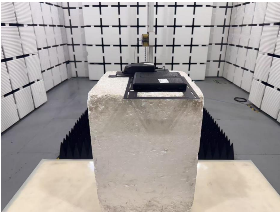
Set-up for Radiated Spurious Emission, Above 1GHz
