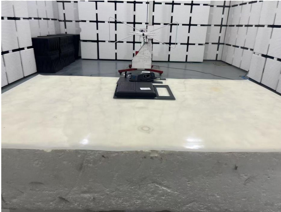
Set-up for Radiated Spurious Emission, Above 1GHz
