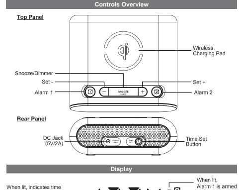
Alarm 1 is armed **-** ① Low Backup Battery Alarm 2 is armed
