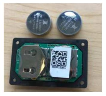
**Step #4**: Insert new batteries with positive sides up (very important) and negative sides against the shields.
