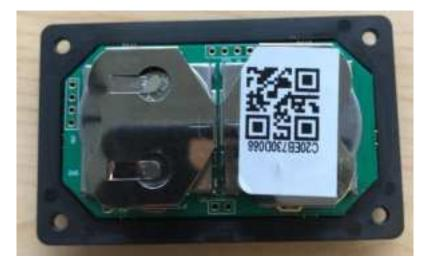
**Step #3:** Remove both batteries.
