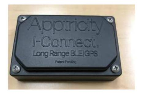
**Step #1:** Remove the 4 screws from the top of the case.
