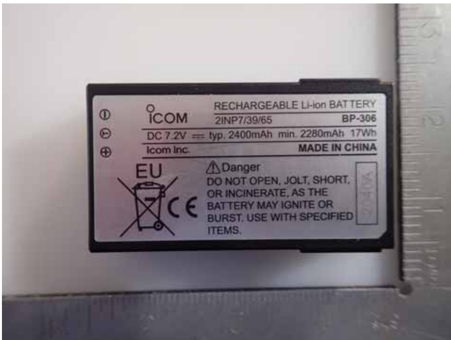
<Li-ion Chargeable Battery (M/N: BP-306, 7.2V, 2400mAh)>
