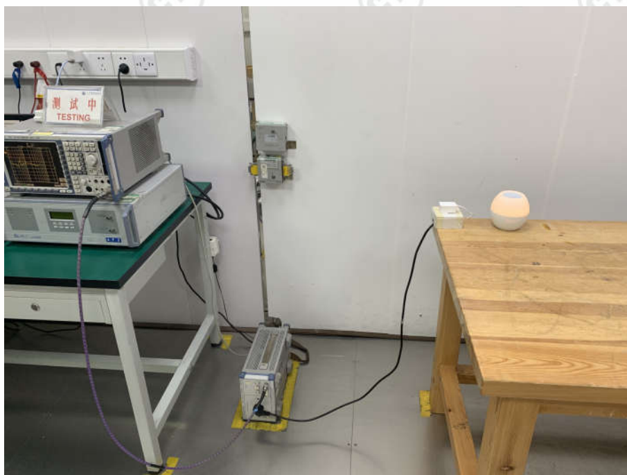
Conducted Emissions Test Setup
