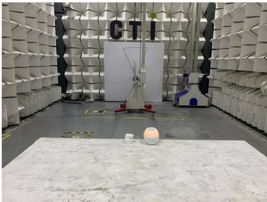
Radiated spurious emission Test Setup-1(Below 1GHz)
