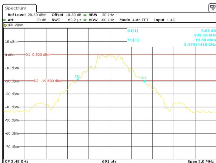
**EDR ( $\pi/4$ -DQPSK): Low Channel**
