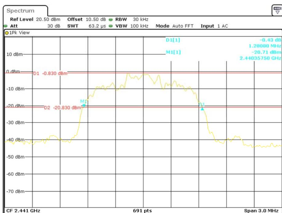
**EDR ( $\pi/4$ -DQPSK): High Channel**
