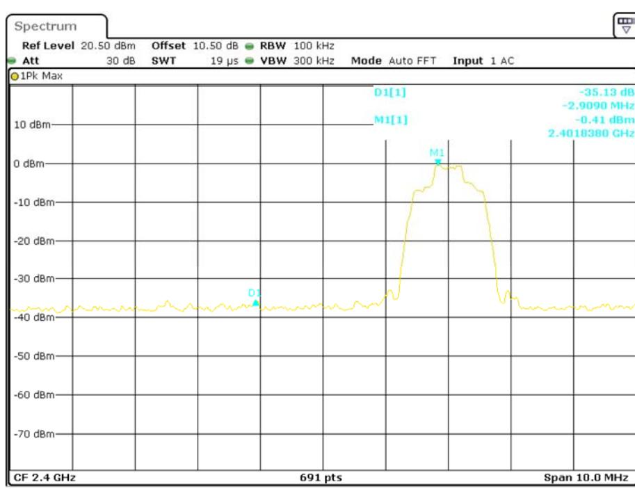
**EDR ( $\pi/4$ -DQPSK): Band Edge-Right Side**
