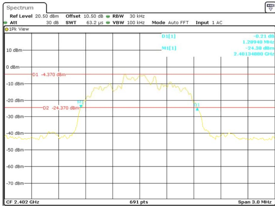
**EDR ( $\pi/4$ -DQPSK): Middle Channel**
