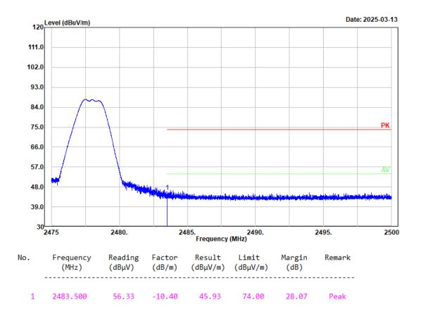
Project No.: 2503R23056E-RF Tester: Mack Huang Condition: PK trace RBW:1MHz; VBW:3MHz; SWT:0.3sec Polarization: Vertical Note: BLE 2M High Channel 2478MHz
