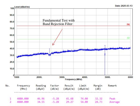
Project No.: 2503R23056E-RF Tester: Mack Huang Condition: PK trace RBW:1MHz; VBW:3MHz; SWT:0.3sec Polarization: vertical Note: BLE 2M Middle Channel 2440MHz
