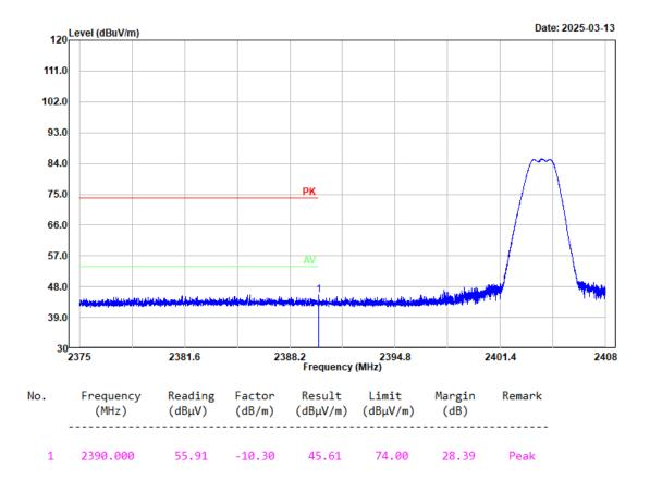
Project No.: 2503R23056E-RF Tester: Mack Huang Condition: PK trace RBW:1MHz; VBW:3MHz; SWT:0.3sec Polarization: Horizontal Note: BLE 2M High Channel 2478MHz
