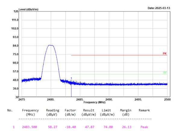
Project No.: 2503R23056E-RF Tester: Mack Huang Condition: PK trace RBW:1MHz; VBW:3MHz; SWT:0.3sec Polarization: Horizontal Note: BLE 2M Low Channel 2404MHz
