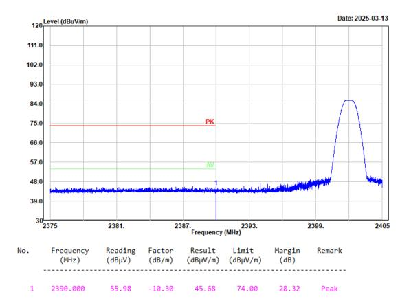
Project No.: 2503R23056E-RF Tester: Mack Huang Condition: PK trace RBW:1MHz; VBW:3MHz; SWT:0.3sec Polarization: Horizontal Note: BLE 1M High Channel 2480MHz
