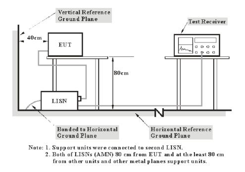
The setup of EUT is according with per ANSI C63.10-2020 measurement procedure. The specification used was with the FCC Part 15.207 limits.
