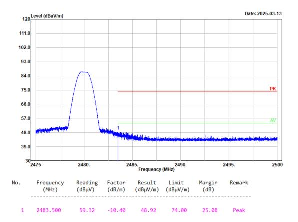
Project No.: 2503R23056E-RF Tester: Mack Huang Condition: PK trace RBW:1MHz; VBW:3MHz; SWT:0.3sec Polarization: Vertical Note: BLE 1M High Channel 2480MHz
