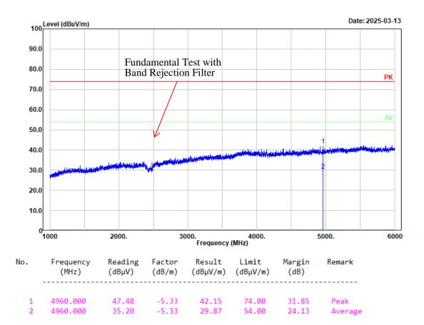
Project No.: 2503R23056E-RF Tester: Mack Huang Condition: PK trace RBW:1MHz; VBW:3MHz; SWT:0.3sec Polarization: vertical Note: BLE 1M High Channel 2480MHz
