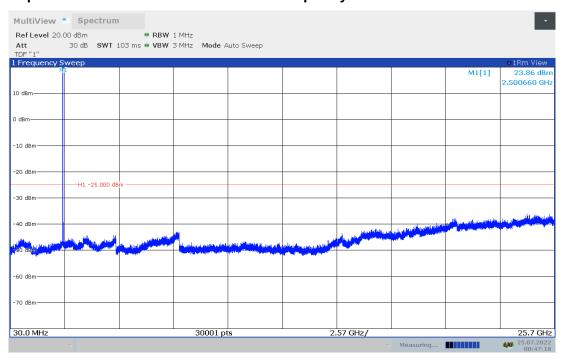
LTE band 41: 30MHz – 26.9GHz Spurious emission limit –25dBm.
