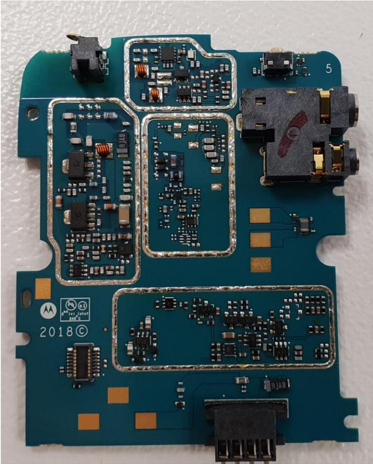
**EXHIBIT 9C - RF board with Shields (Bottom)**
