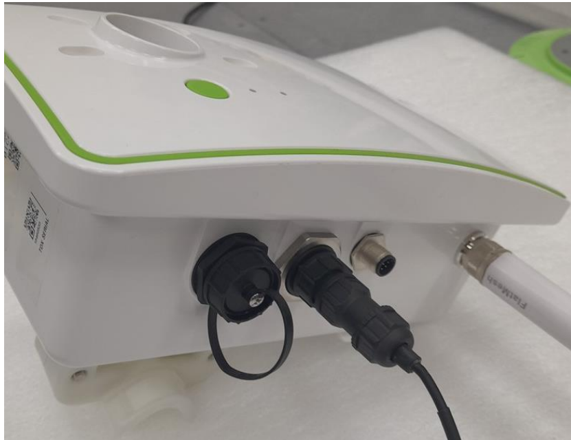
Figure 2.3: Power Connector on Camera Hub near FlatMesh Antenna.
