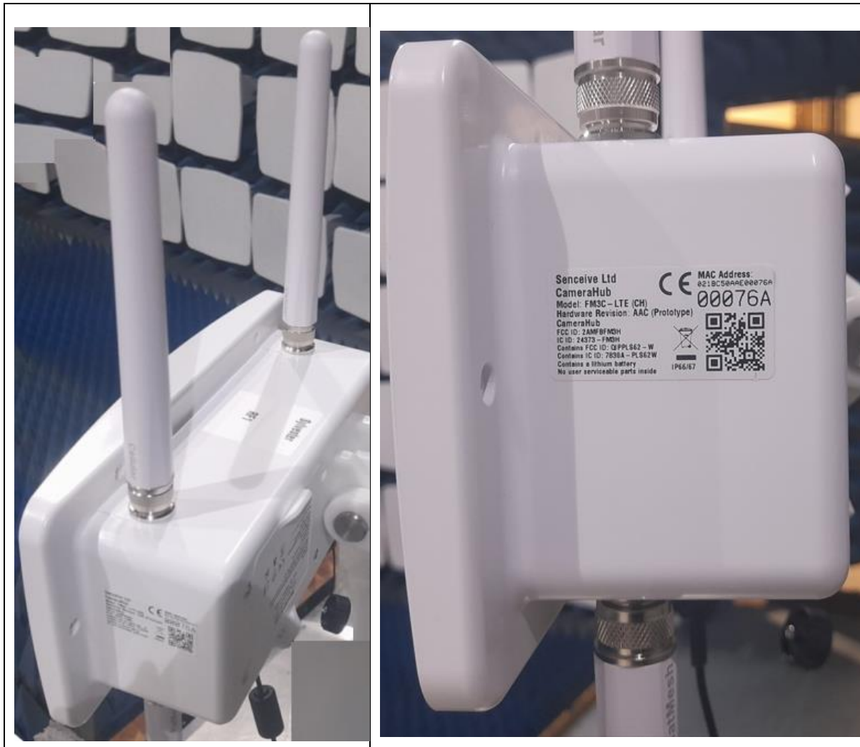
Figure 2.5: Antennae fitted to Camera Hub (top view displaying the 2 No. Cellular Antennae) and (side view displaying the connected N-Type FlatMesh 2.4GHz antenna on the bottom side of the Camera Hub)
