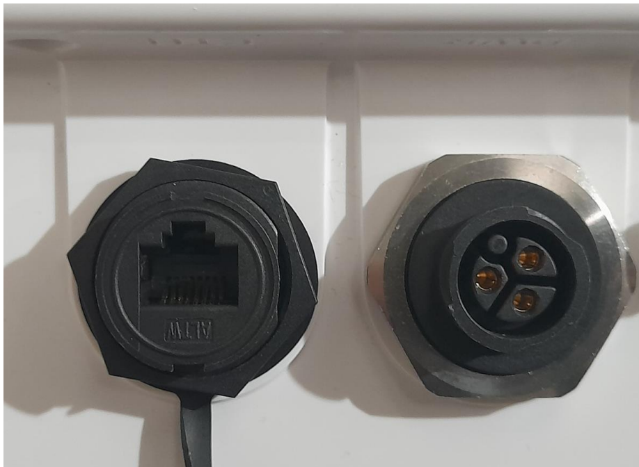
Figure 2.6: Ethernet connection point on the Camera Hub
