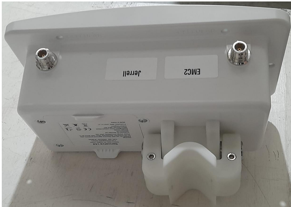
Figure 2.1: Camera Hub Rear Bracket for Pole Mounting
