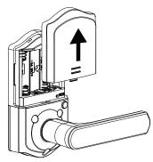
Do not load batteries until the lock is completely installed.
