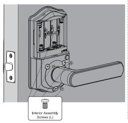
Insert 4 AA Alkaline batteries and put on the Battery Cover.
