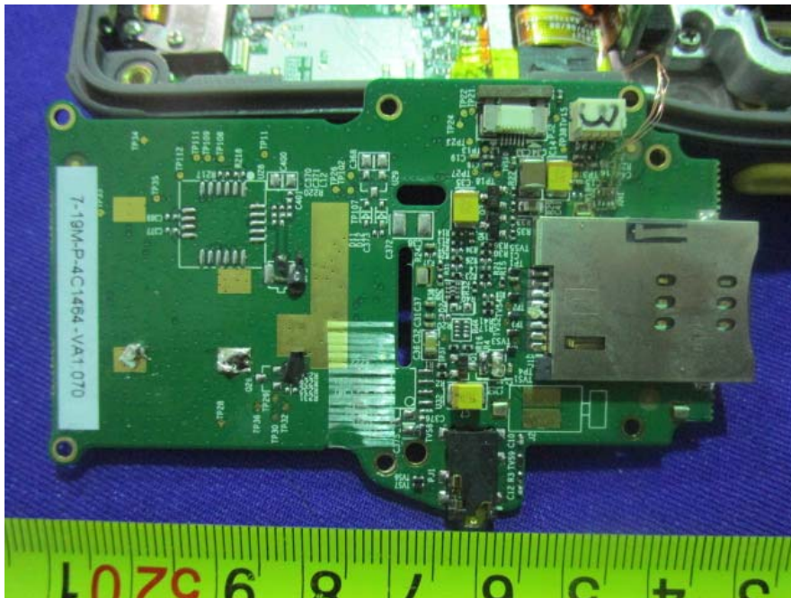
EUT – Sub Board 1 Top View
